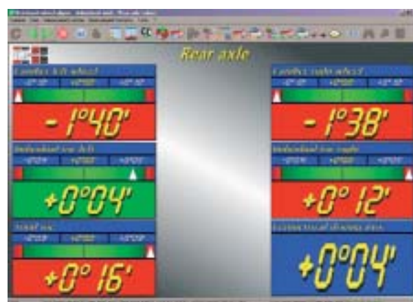
Rear-axle measured-value display: Full information available at a glance.
